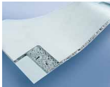
Aluminium Foam Sandwich (AFS): As its name implies, outer layers of aluminium or steel sheet alloyed to an aluminium foam core
